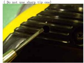
$2\ \mbox{Remove}$  one side of saddle panel on which no switch is located.
