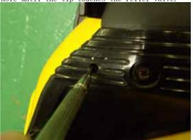
7 Move the precision screwdriver sideway to slide the relief valve. By this operation, air gets into the head assembly to take the pressure equilibrium.
