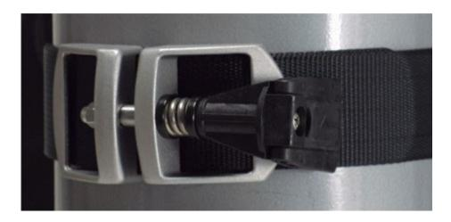
Tighten the belt by turning the knob until spring is fully compressed.
