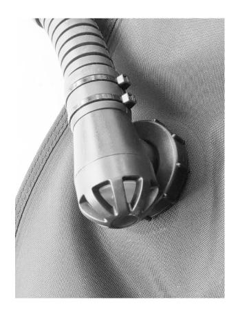
The Elbow dump sits on the left-hand shoulder. To operate the valve, pull the inflator unit attached to the corrugated hose. The inflator pulls on a cable running through the hose to operate the valve.
